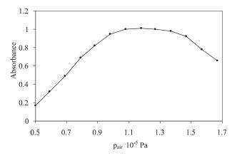
Fig. 3. Correlation between absorbance of strontium and air pressure ( $p_{C_3H_2} = 2.45 \cdot 10^4$  Pa,  $c_{sr} = 1 \mu g/ml$ ).
