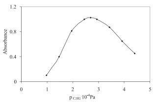
Fig. 2. Correlation between absorbance of strontium and pressure of acetylene ( $p_{air} = 1.18 \cdot 10^5 \text{ Pa}$ ,  $c_{Sr} = 1 \ \mu\text{g/ml}$ ).
