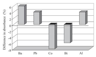
Fig. 8. Effect of the concentration of Ba, Pb, Co, Bi and Al ions on the analytical signal of Sr (Sr:M = 1:2,000).
