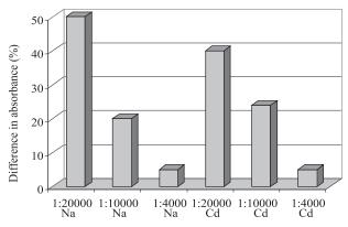
Fig. 7. Effect of the concentration of Na and Cd ions on the analytical signal of Sr.
