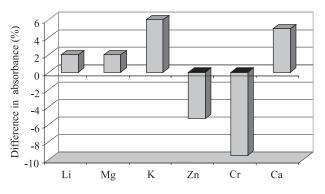
Fig. 4. Effect of the concentration of Li, Mg, K, Zn, Cr and Ca ions on the analytical signal of Sr (Sr:M = 1:20,000).
