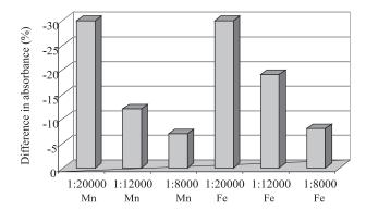
Fig. 6. Effect of the concentration of Mn and Fe ions on the analytical signal of Sr.
