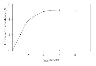
Fig. 1. Correlation between absorption signal and hydrochloric acid ( $p_{air} = 1.18 \cdot 10^5$ ,  $p_{C2H2} = 2.45 \cdot 10^4$  Pa,  $c_{Sr} = 1 \mu g/ml$ ).
