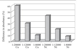
Fig. 5. Effect of the concentration of Cu and Ni ions on the analytical signal of Sr.
